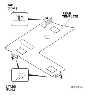
8. Align the two tabs of the rear template onto the edge of the left rear door as shown.
