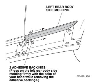
18. Using the rubber roller, apply firm pressure while rolling to set the adhesive. Apply firm pressure especially at the ends.
