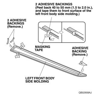
12. Align the left front body side molding with the front and middle templates, and install the left front body side molding on the left front door.
