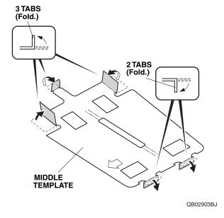
5. Align the middle template onto the left front and rear doors as shown.
