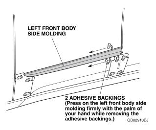
14. Using the rubber roller, apply firm pressure while rolling to set the adhesive. Apply firm pressure especially at the ends.
