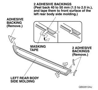
Align the left rear body side molding with the middle and rear templates, and install the left rear body side molding on the left rear door.
