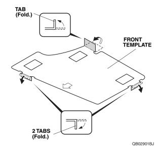
2. Align the two tabs of the front template onto the left front door as shown.
